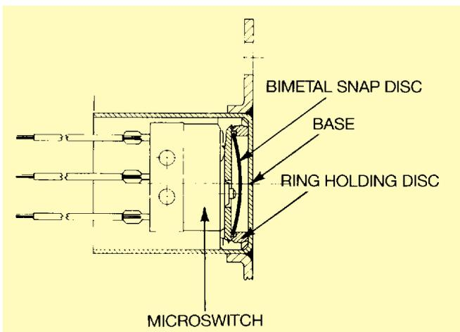
Figure 3: Bimetallic disc
