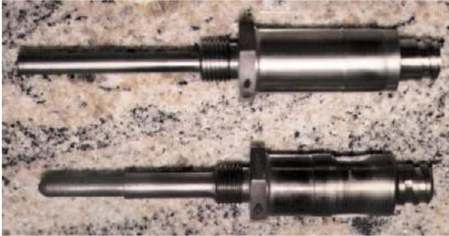
**Figure 5: Shrouded versus non-shrouded rod and tube**
